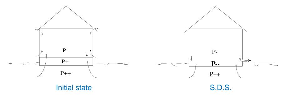
To generate a slight depressurization of basement compared to indoor environment with low extract flow
