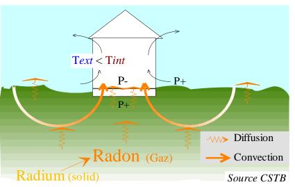
Main process: convection generated by depression due to stack effect and wind
