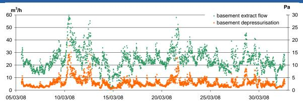
Evolution of basement extract flow  $(Q_{SDS})$  and basement depressurisation
