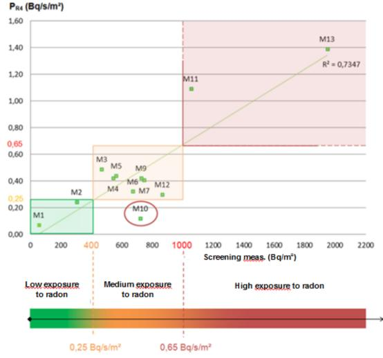
P<sub>Rn4</sub> < 0,25 Bq/s/m<sup>2</sup> → low exposure to radon
