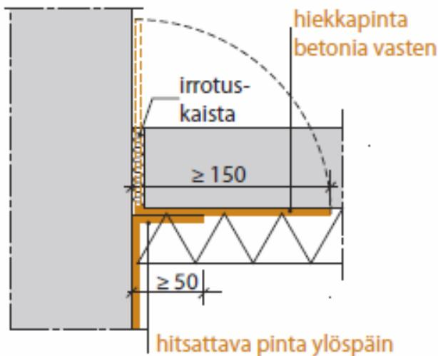
Bitumen felt welded to the surface of the foundation wall (concrete)
