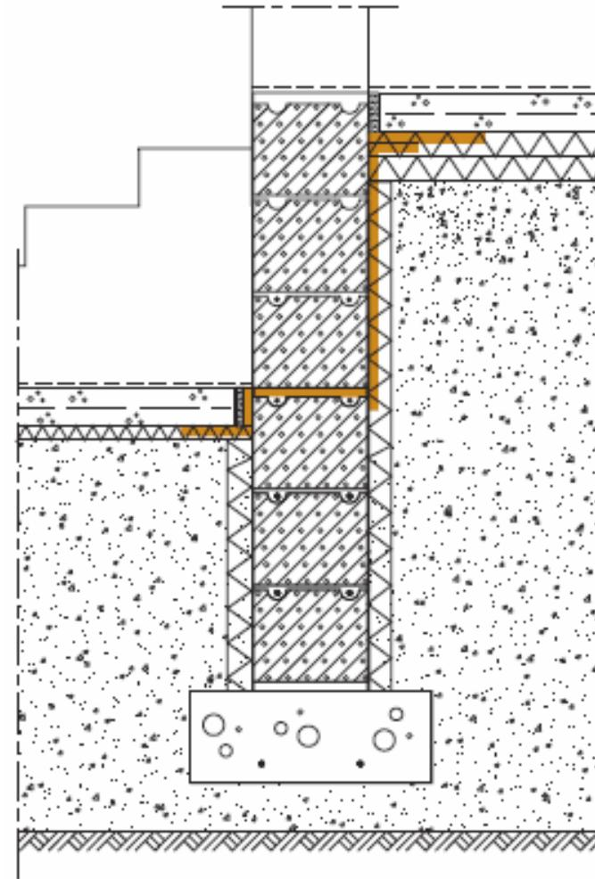
Stepped base floor – three strips of bitumen felt welded together
