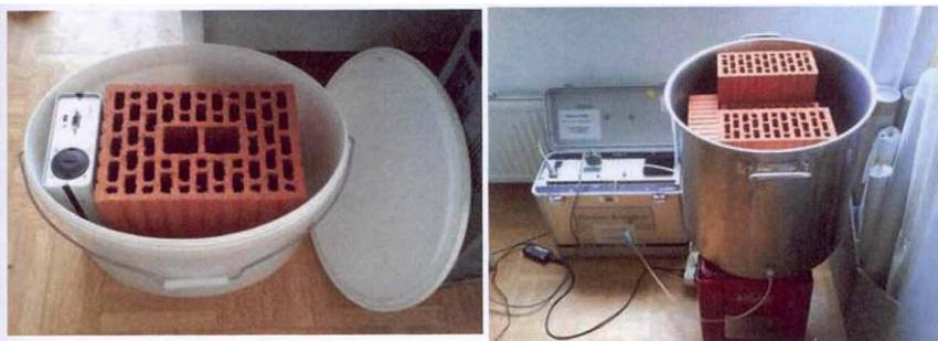
Abbildung 42: Links: interner Radonmonitor (Radon Scout)
